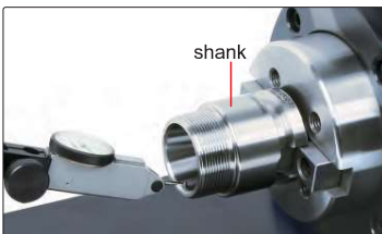
measure radial runout of shank
