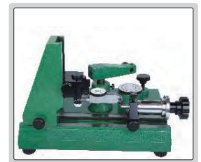
inspect accuracy of test indicators
